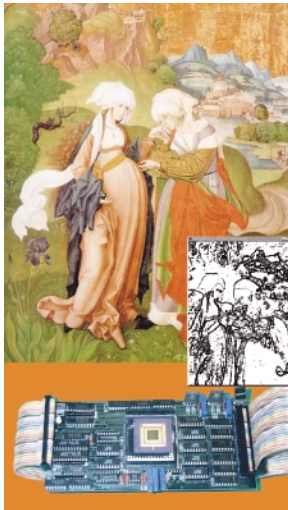
A new analogic cellular supercomputer system, a visual microprocessor, performs a trillion operations per second.
