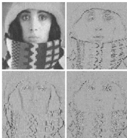
Decomposition of a grey-scale image by a morphological wavelet (max-lifting scheme). The original image is shown at the left and its decomposition into four subbands at the right.
