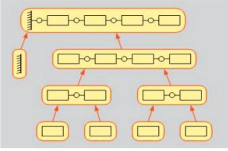
The construction of a rigid-body system from its component bodies by recursive pairwise assembly. The new divide-and-conquer algorithm constructs the equations of motion in the same manner.
