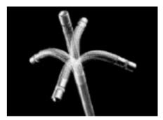
Figure1: The motion of the tip of the endoscope.
