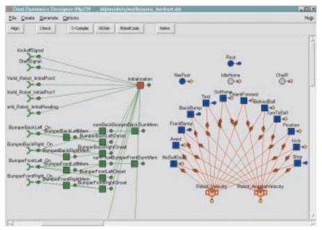
Figure 2: DD-Designer with a graphical specification of a Dual Dynamics behavior system.
