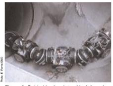
Figure 2: Guided by the data of its infrared and image sensors, MAKRO can automatically perform turns and overcome steps. The robot can operate in sewer pipes of diameters within a range of 300 to 600 millimeters.
