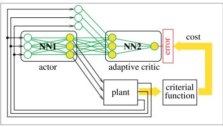
Structure of the adaptive critic controller based on artifical neural networks.
