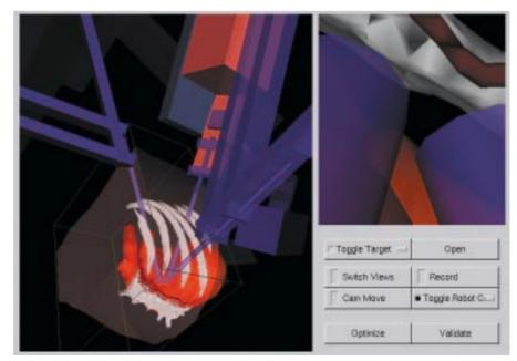
The software designed in the Chir team for the planning and simulation of surgical interventions. Upper right: the endoscopic view, left: the external positionning the robot in the thoracic cage.
