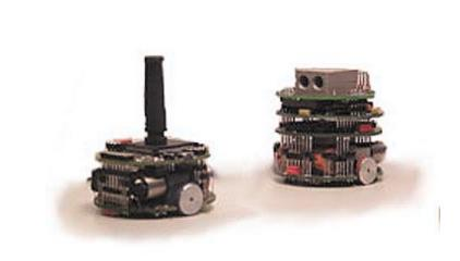
The predator and prey robots consist of two Khepera robots. The predator is equipped with a vision module while the prey has a maximum available speed set to twice that of the predator. Both species were also provided with eight infrared proximity sensors (six on the front side and two on the back). Khepera has been developed at the Laboratory of Microcomputing of the Swiss Federal Institute of Technology (EPFL) in Lausanne.
