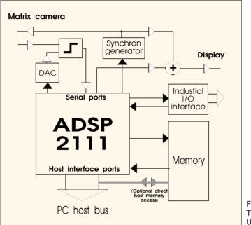
Figure 1: The layout of the UltraGrab card.
