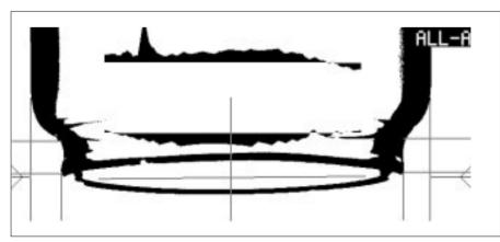
Figure 3: Processed image of the glass tube collar.
