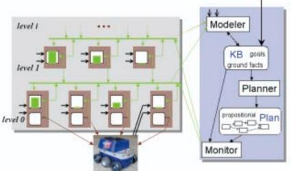
Schema of the DD&P robot control architecture. See text for explanations.
