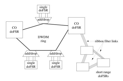
Figure 1: An example of heterogenous doFSR network architecture.
