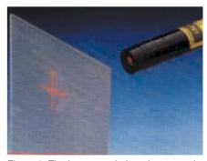
Figure 3: The laser crosshair projector used for MAKRO robot orientation in the sewer.
