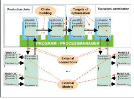
Figure 2: Hybrid modelling and optimisation of process chains by ProcessManager
