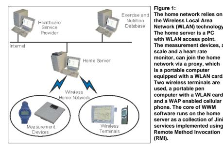
Figure 1: The home network relies on the Wireless Local Area Network (WLAN) technology. The home server is a PC with WLAN access point. The measurement devices, a scale and a heart rate monitor, can join the home network via a proxy, which is a portable computer equipped with a WLAN card. Two wireless terminals are used, a portable pen
