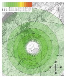
Figure 1: Isoconcentration zones in circle representation for the planned turbine testing plant, for the most frequent meteorological condition (9,7° C air temperature, 2 m/s wind speed, B stability indicator), NO<sub>X</sub>, emission: 362,2 kg/h, imission limit value: 150  $\mu$ g/m3.
