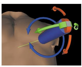
The virtual transducer is positioned on the thorax model and can be swept, tilted, and rotated by dragging at the three touch-sensitive areas (blue, red, and green).
