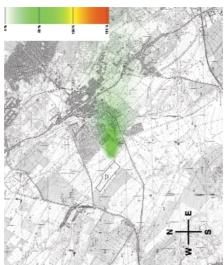
Figure 2: Concentration tail in W winddirection for the planned turbine testing plant, for the critical meteorological condition ( $35^{\circ}$  C air temperature, 5 m/s wind speed, B stability indicator), NO<sub>X</sub>, emission: 362,2 kg/h, imission limit value: 150 µg/m3.
