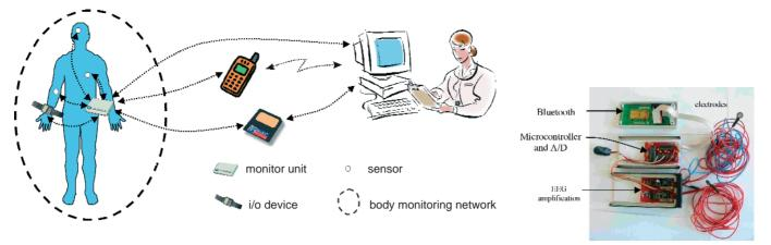
Figure 1: Overview of the Body Monitoring System.
