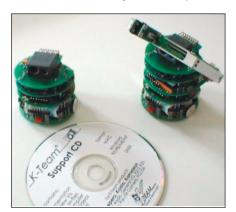
Figure 1: The Khepera robots.
