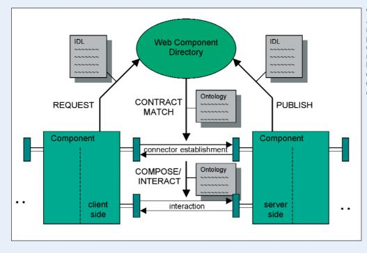
Web Component Life-Cycle. A component request might by matched by a server component published in a Web component directory. Successful matching results in direct communication between client and server component to establish a connector for service invocation and reply.
