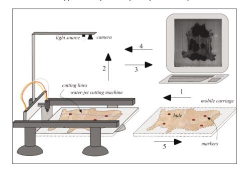
Figure 1: The Cutting System.
