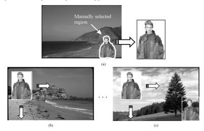
Figure 2. *Example for image retrieval with dynamic extracted features: (a) Creation of a region of interest; (b) Search for the region in an unsuitable image; (c) Person found in another image by template matching*
