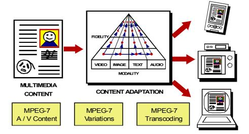
Figure 2 Figure 2: Illustration of Universal Multimedia Access (UMA) in which the appropriate variations of the audio-visual programs are selected according to the capabilities of the terminal devices. The MPEG-7 transcoding hints may also be used to further adapt the programs to the devices.
